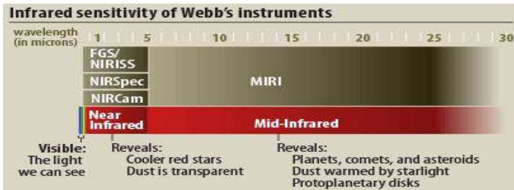
Fig 2.5:- range scale of NIRCAM (0.6 – 5 microns)
