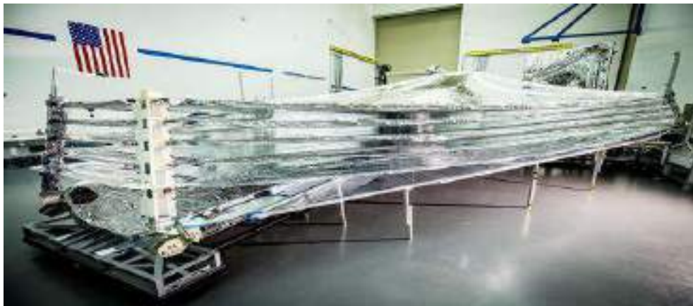
Fig 3.3:-5 layers of sunshield
