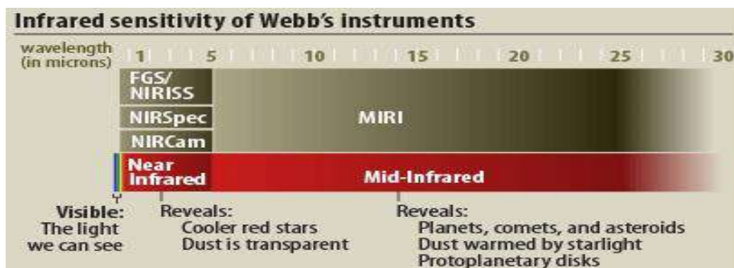
Fig 2.3:- range scale of NIRSpec ( 0.6 – 5 microns)
